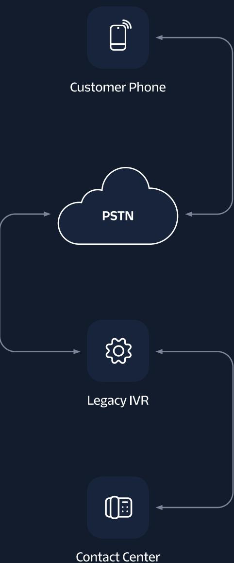
Twilio's cloud-based approach to IVR makes it easy to augment or replace your traditional IVR with one that offers cloud scalability and easy customization. The diagram shows how Twilio's cloud-based IVR can replace your legacy IVR system, while retaining key components like your phone number and contact center for a seamless transition.
