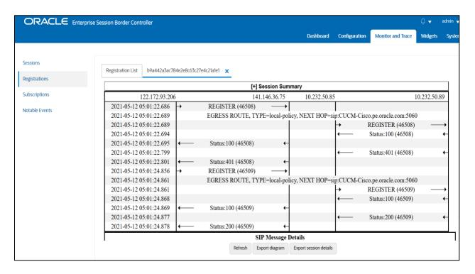
3. Make Call from Cisco Remote user to the Twilio Elastic Sip Trunk user and check the call flow. Now, there will be 2 call legs (hair pinned call) as the call reaches Cisco CUCM first and then reaches Twilio trunk user after that as given below.
