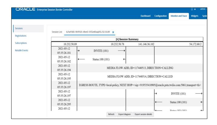
4. Make Call from the Twilio Elastic Sip Trunk to Cisco User and check the call flow. The calls flow from 141.146.36.102 (Twilio Elastic SIP Trunking Interface) to 10.232.50.78 (Cisco SIP Interface) and the call reaches the Cisco user after that.
