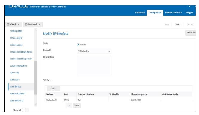
Once sip-interface is configured – the SBC is ready to accept traffic on the allocated IP address.
