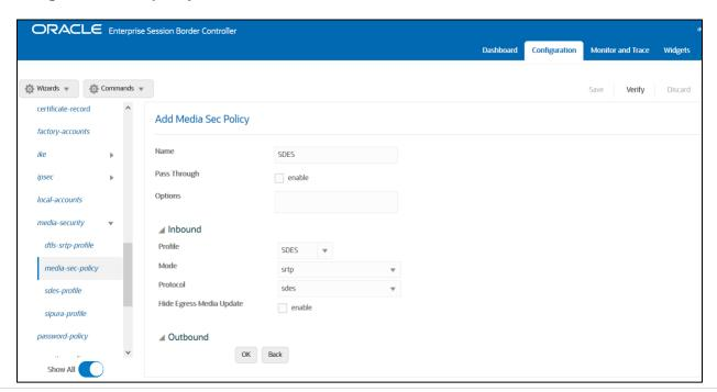
Similarly, Create Media Sec policy with name RTP to convert srtp to rtp for the Cisco side which will use only TCP/UDP as transport protocol. **Assign this media policy to the Cisco Realm.**
