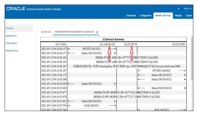
5. Make Call from Twilio Elastic Sip Trunk user to Cisco Remote user and check the call flow. Now, there will be 2 call legs (hair pinned call) as the call reaches Cisco CUCM first and then reaches Cisco Remote user after that as given below.
